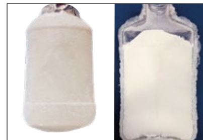
Fig. 2 - Above is represented the pressure rise inside 5 L bottles with different wall thickness during freezing. The thinner bottle was able to release the internal pressure by substantial deformation and a convex bottom (at the bottom left). The thicker bottle deforms slightly but the internal pressure was kept high (at the bottom right).
